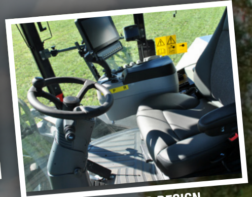
SUPERIOR CAB DESIGN Large spacious cab featuring a premium leather seat with cooling/heating features. New standards for visibility allow the entire boom to be seen with uninterrupted forward vision.
