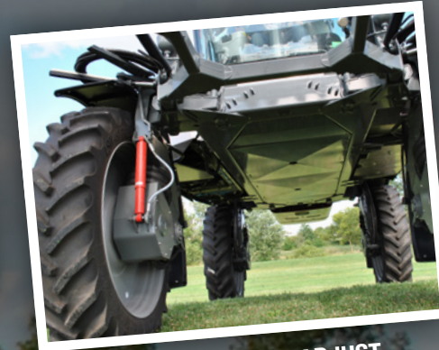
HYDRAULIC TRACK ADJUST The RUBICON axle track width can be adjusted, on-the-run, from 118" to 157". The integrated air-ride suspension provides superior ride and performance.
