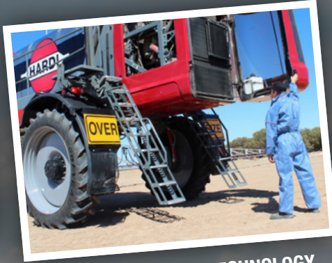
ADVANCED ENGINE TECHNOLOGY RUBICON is powered by Cummins® 8.9L QSL 9, Tier 4F Engine 380 HP
