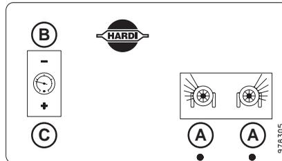
1. ON/OFF switches **A** are set to ON position.
