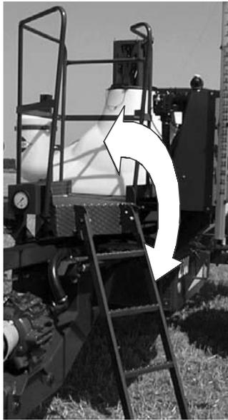
**NOTE!** Always unfold the ladder before driving.
