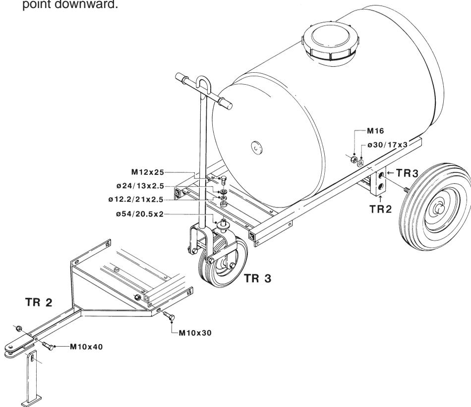
4. Bolt unit on frame (only PU).
