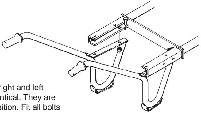
2. Note: On KS 100 right and left handle are not identical. They are fitted in widest position. Fit all bolts in pump unit/tank frame/handle before tightening the bolts.
