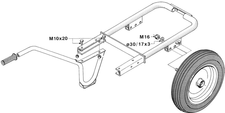
3. On TR3 use upper hole in tank frame - fit nose wheel.
