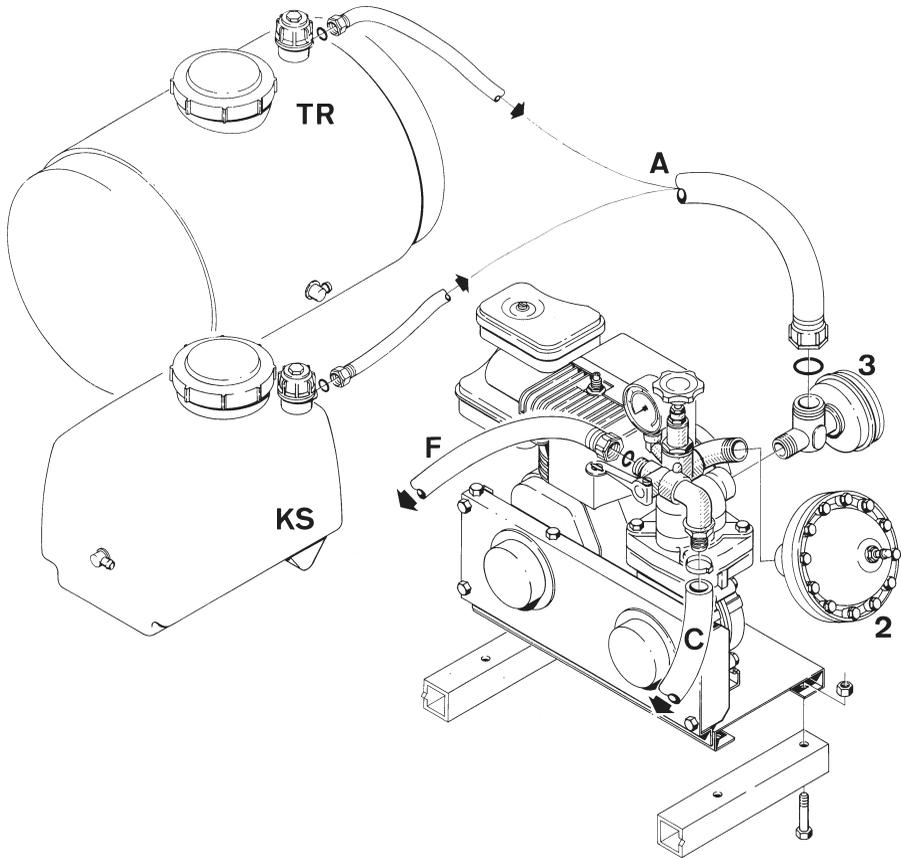
5. Check that all hoses are fitted according to the diagram. PRES-
