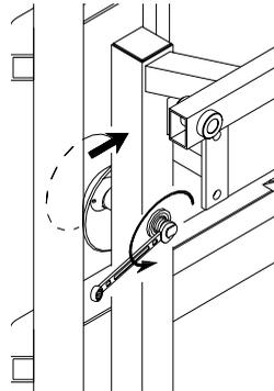
4. Make sure that the contact surface between the eccentric axle and liftwagon is free of grease and paint.
