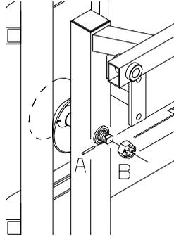
2. Turning the eccentric axle clockwise will decrease the gap between the wheel and the lift. Use a spanner.
