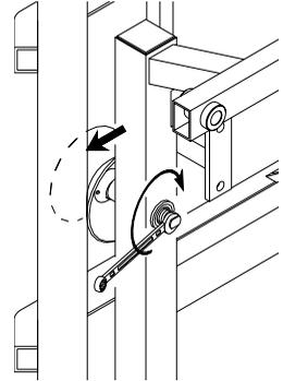
3. Turning the eccentric axle counter clockwise will increase the gap between the wheel and the lift. Use a spanner.
