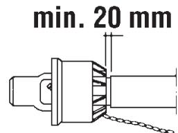
6. Fit the shaft to tractor and sprayer pump.
