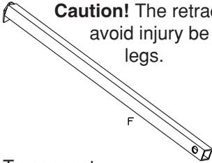
**Caution!** The retractable support legs are spring-loaded - to avoid injury be careful during folding/unfolding of the support legs.
