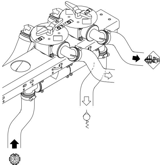
If all the green pressure valves are closed the safety valve will open inside the tank.
