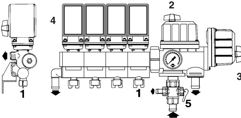
1. Adjustment screw for pressure equalization
