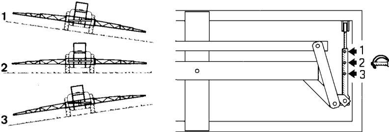
When driving on slopes the boom can be slanted in order to keep the trapeze effect. At delivery the boom is locked in pos. **2** which is used when driving on horizontal grounds. Hydraulic slanting equipment can be supplied as optional extra.
