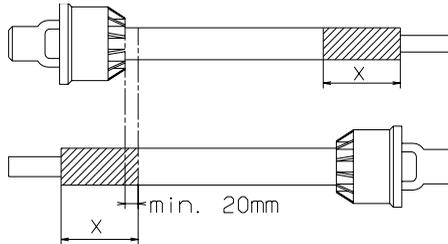
**NOTE:** The shaft must always have a minimum overlap 150 mm.
