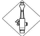
**NOTE:** Turn handle towards EC-operating unit **before** turning away from Fast Filler in order to avoid peak pressure blowing the safety valve!
