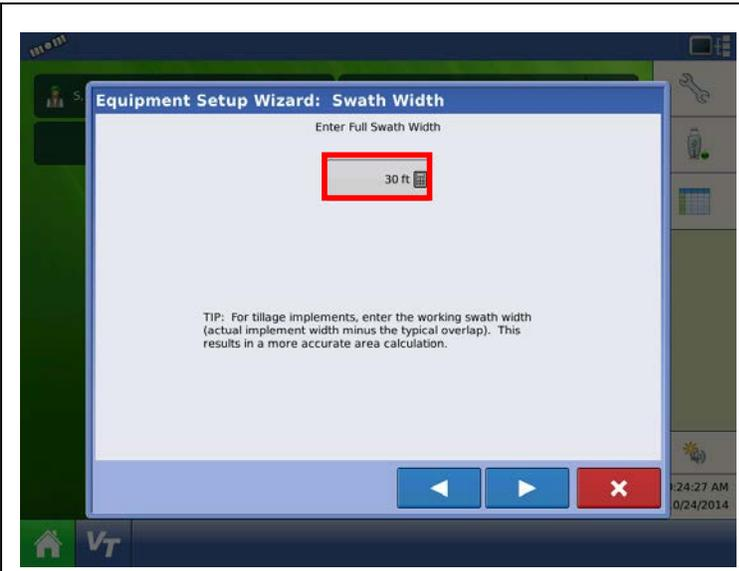
Next, enter in the swath width of the boom. Press the calculator to enter in the correct value.
