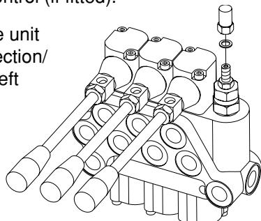
**NOTE:** The hydraulic system requires a minimum oil pressure of 130 bar, max. pressure 160 bar and an oil capacity of approx. 3 litres. After having operated the boom and the system has been filled with oil, check tractor hydraulic oil level and top up if necessary.
