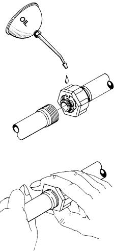
The O-ring is lubricated **ALL THE WAY ROUND** before fitting on to the nozzle tube. Use non-mineral lubricant.
