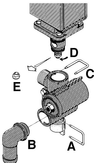
Remove the clip **C** and lift the EC-motor housing off the valve housing. Then unscrew the screw **D** and replace the valve cone **E**. Reassemble in opposite sequence.
