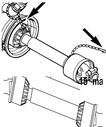
6. Fit the shaft to tractor and sprayer pump. **NOTE:** Female part towards tractor. Fit the chains to prevent the protection guards to rotate with the shaft.
