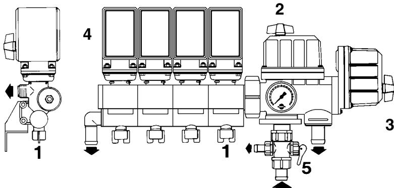
1. Adjustment screw for pressure equalization
