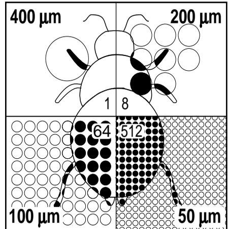
Halving one 400 mm drop produces 8 drops of 200 µm. With these smaller drops, it is possible to cover about twice the area.
