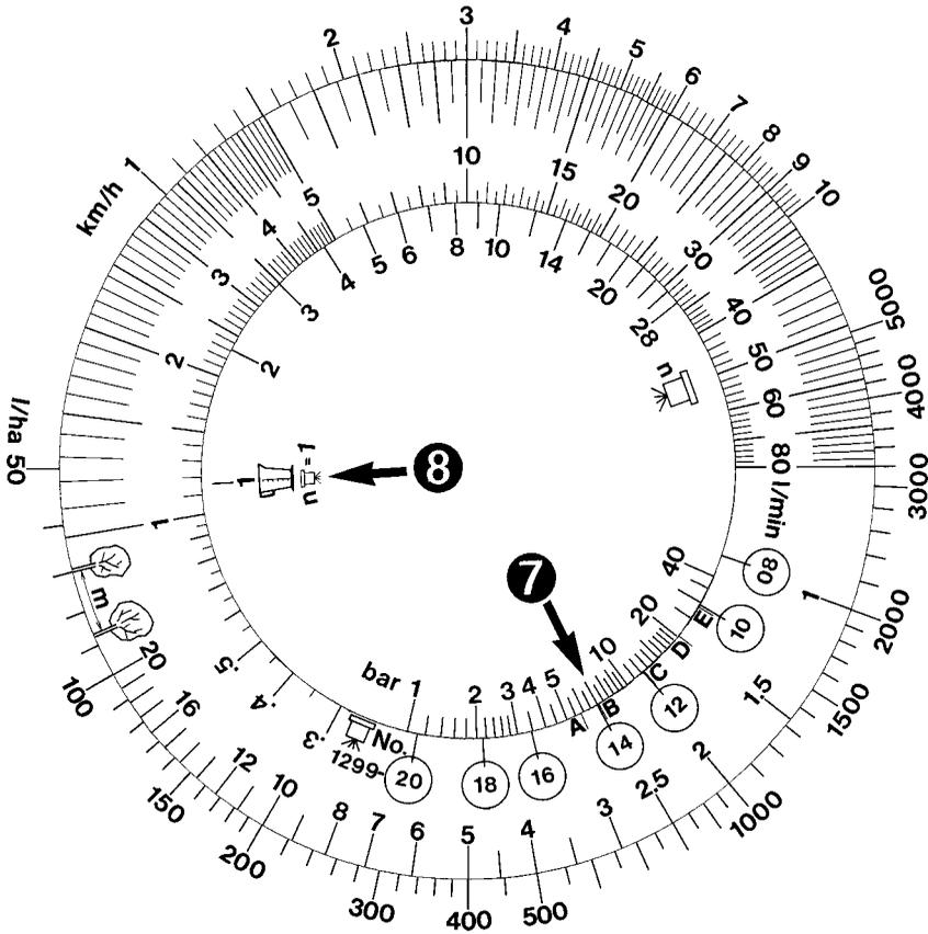
Align the nozzle sizes one by one with 7.1 bar
