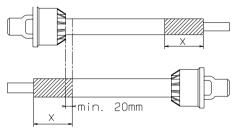
**NOTE:** The shaft must always have a minimum overlap of 150 mm.
