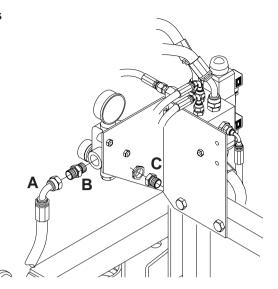
To convert sprayer for closed centre hydraulics:
