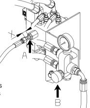
**NOTE:** If the boom has difficulty in unfolding, increase the oil flow to the blower by turning valve **B** on the blower.
