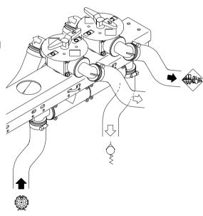
"O" (closed). When spraying is to resume, select the Self-Cleaning Filter/operating unit. The other handles are turned to "O".
