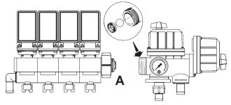
union nut A and pull the valve away from the distribution valves.
