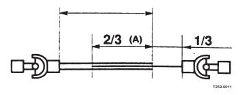
4. The two parts are shortened equally. Use a saw, and file the profiles afterwards to remove burrs.
