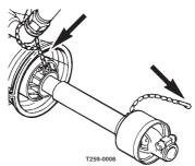
8. To ensure long life of the transmission shaft, try to avoid working angles greater than 15°.
