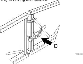
5. Unfold the left side fold of the boom and use the same procedures as described in point 4.
