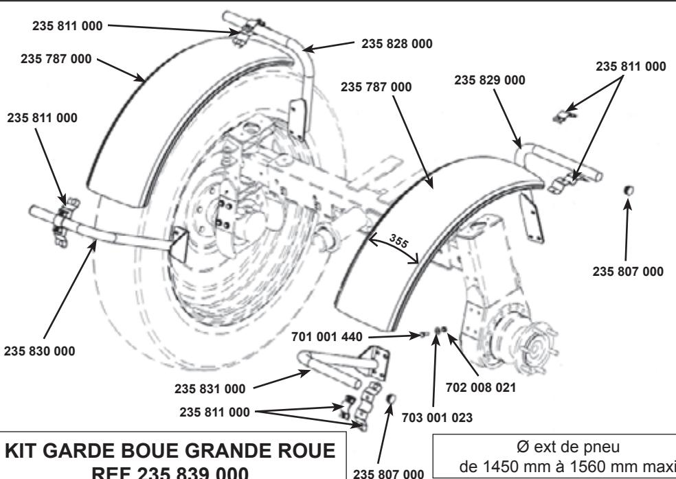
Tyre's width less than 400 mm
