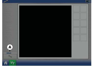
If there are multiple ISO implements connected, press the VT button v<sub>T</sub> to toggle between Working Sets.
