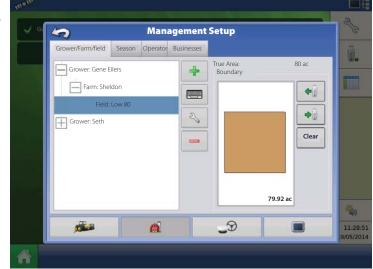
Edit an existing name of a Field by highlighting that name and pressing button.
