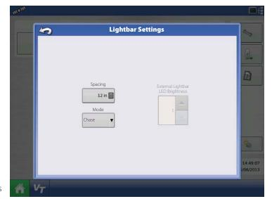
external lightbar. The number 1 is the dimmest setting and 10 is the brightest. Default setting is 5.
