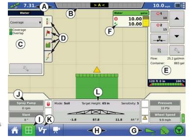
The task bar (H) displays buttons relating to various functions of the display. These buttons and status indicators include:
