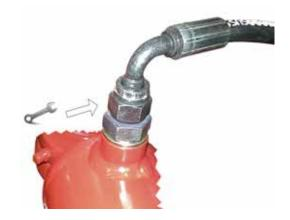
A DANGER! A hydraulic hose or joint leaking or coming apart with the oil under pressure can cause severe injuries to persons standing nearby! The oil can be very hot, around 176° F (80 °C), and the oil streaming out can penetrate human skin. Risk of burns on the skin, internal injuries and facial injuries.
