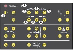
6. If equipped with Dual Fold boom, push switch (7) to fold 2nd outer sections in to reduced working width.
