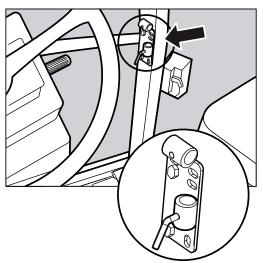
The supplied tractor pillar bracket (A) has a hole spacing of 3.9 in. (100 mm) and 4.7 in. (120 mm), which fits most tractors. Threaded mounting holes may be hidden behind front corner cover. Check the tractor's instruction book for information regarding attachment points.
