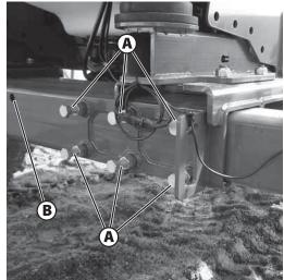
9. Re-tighten bolts and wheel bolts to specified torque after 8 hours of work.
