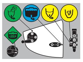
5. Measure the correct amount of powdered chemical and sprinkle it into the hopper as fast as the transfer device can flush it down. The TurboFiller suction valve must be open for at least 20 seconds after the chemical is no longer visible in the hopper in order to completely empty the transfer hoses into the main tank.
