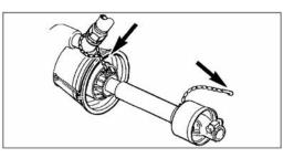
To ensure long life of the transmission shaft, try to avoid working angles greater than 15°.
