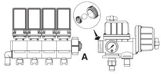
and pull the valve away from the distribution valves.
