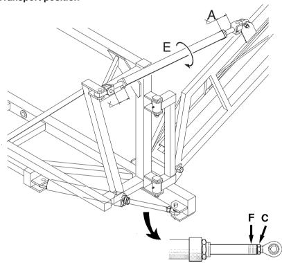
The boom is to be adjusted so that boom movement is not possible during transport.
