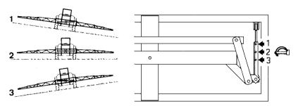
When driving on slopes the boom can be slanted in order to keep the trapeze effect. At delivery the boom is locked in pos. **2** which is used when driving on horizontal grounds. Hydraulic slanting equipment can be supplied as optional extra.
