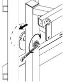
Turning the eccentric axle counter clockwise will increase the gap between the wheel and the lift. Use a spanner.
