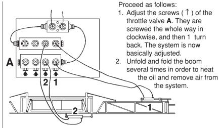
3. Set the adjustment screws on the throttle valve until the individual rams run with the speed wanted (clockwise = less speed).
