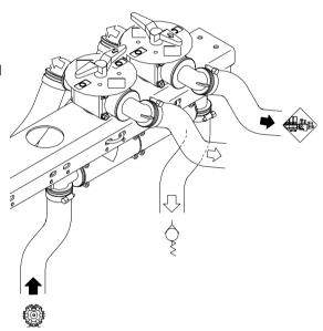
"O" (closed). When spraying is to resume, select the Self-Cleaning Filter/operating unit. The other handles are turned to "O".
