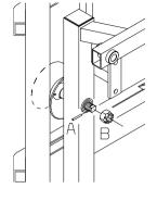
2. Turning the eccentric axle clockwise will decrease the gap between the wheel and the lift. Use a spanner.
