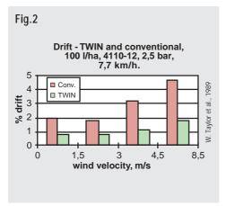
**Fig. 2.** The importance of air assistance in controlling drift over a wide range of wind velocities is critical to the TWIN. Note that volume of airborne drift from TWIN air assisted sprayer in a high wind speed of 8,5 m/s - is as low as the drift from the conventional sprayer at optimum spraying conditions (1,5 m/s). The tests were carried out over bare ground/ short cut grass.
