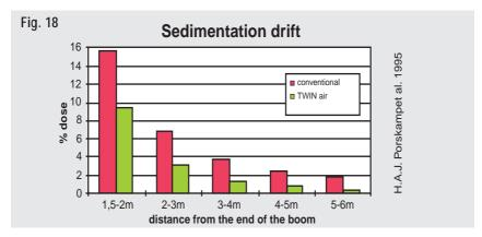
**Fig. 18.** "Dosing" on the downwind out of the treated area. TWIN has halved the deposit out of the target area, compared to spraying with a conventional sprayer. Both systems applied 150 l/ha of Fine Sprays (4110-12, 3 bar).
