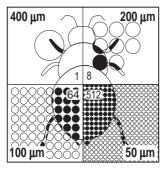
**Fig. 3.** Each square represents equal water quantities but atomised into four different droplet sizes. The smaller the droplet size - the better the coverage. The volume rate can be reduced significantly - generally by 50 % of conventional use, sometimes more, because the small droplets are much more efficient for coverage - and with the TWIN air assistance they are safe to use.
